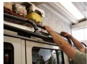
First step is to fit 2 main aches in right position, then link with orizontal tubes and plates on roof top (in case of SW model, no necessary if with softop), linking RH to LH with small top arch.
