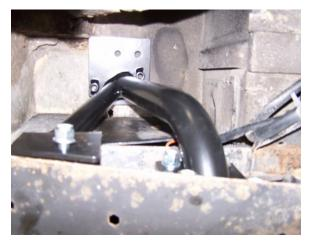
REAR RH-LH CHASSIS BRACKETS - Fit from crossmember to up body.
