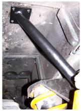
MIDDLE RH-LH CHASSIS BRACKETS - Fit from shocks absorber bracket to up body central.
