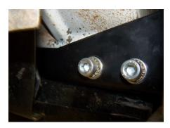
Front bracket to chassis (only for 02102 roll cage) is fitted inside of body to create first fitting point to chassis; right position of bracket create position fo 4 holes on fender to fit outer arm of cage.
